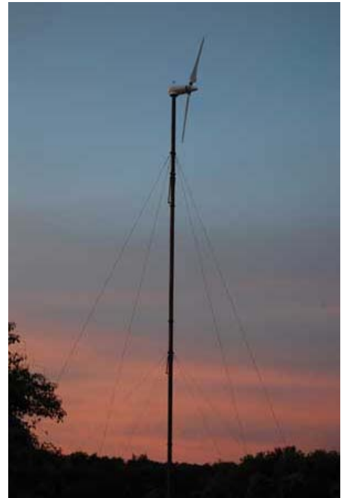
Aerostar's wind turbines are stall regulated, a feature enabled by the Viterna model.
